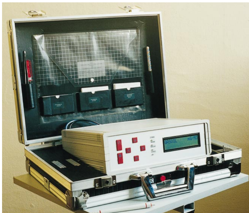
Portable gas-analyzer for air pollution control: detection limit, 1–10 ppm.
