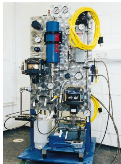
The UniCarb™ process uses carbon dioxide to replace organic solvents in spray coating systems.
