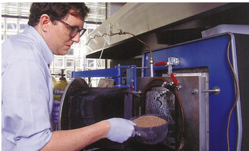
Raw macadamia nut shells being placed in a special oven where they will be carbonised and activated at temperatures above 800 °C. USDA-ARS photo by Scott Bauer
