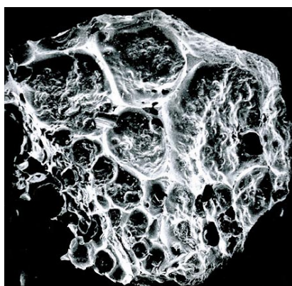
Scanning electron micrograph showing the effect activation has on the gross structure of nut shell carbon granules. While it is impossible to see active micro- and meso-pores, the large pits are significant evidence of gasification. USDA-ARS photo by Chris Toles.
